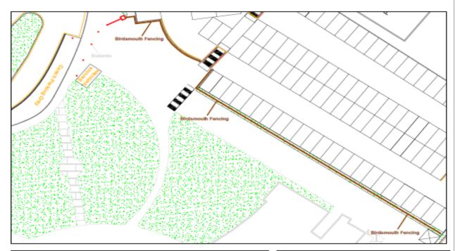
Installation of access control Barrier to control overflow parking, bollards and single rail timber fence following the kerb line to secure area and prevent parking on pavement. Inclusion of zebra crossing for pedestrians safety across the access road.
