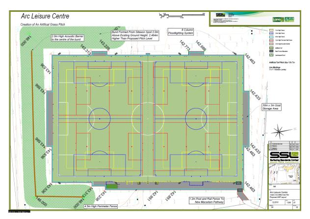
In accordance with environmental health recommendations, and in order to protect the amenity of adjacent residents from potential noise and disturbance, amendments have been received to install a 2m high acoustic fence on top of the proposed landscape bund, providing a screen to the south, and part of the eastern boundary of the proposed pitches. The fence shall have a total length of 110m.
