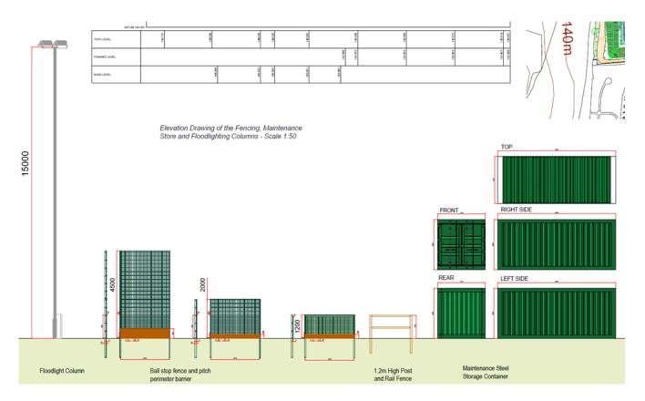
Surrounding the entire perimeter of the artificial pitches will be 4.5m high ball stop fencing, and there will be a 1.2m pitch perimeter barrier along part of the eastern side of the pitch, the appearance of which are identified on the plan above. A dark green, steel maintenance storage container will be built adjacent to the pitch, inside of the perimeter fencing.
