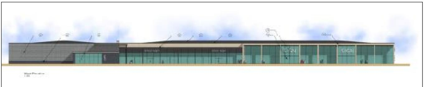
The design of the buildings involves extensive glazing to the frontages, with additional glazing on the Cartwright Lane side of the food and drink 'pod'. These are to be clad in a mix of blue brick, stone rainscreen cladding (buff) and grey ceramic tile. The rear elevations (north and east facing) are microrib composite cladding panels laid vertically and randomly of different shades of green and buff to break up these extensive elevations.
